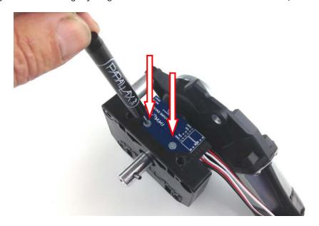
This completes the assembly of one of the drive units. Duplicate what you just accomplished and when you're finished the result is two separate motor drive units that are mirror images of each other—one for the right side and one for the left side of your robot platform, as shown here.
