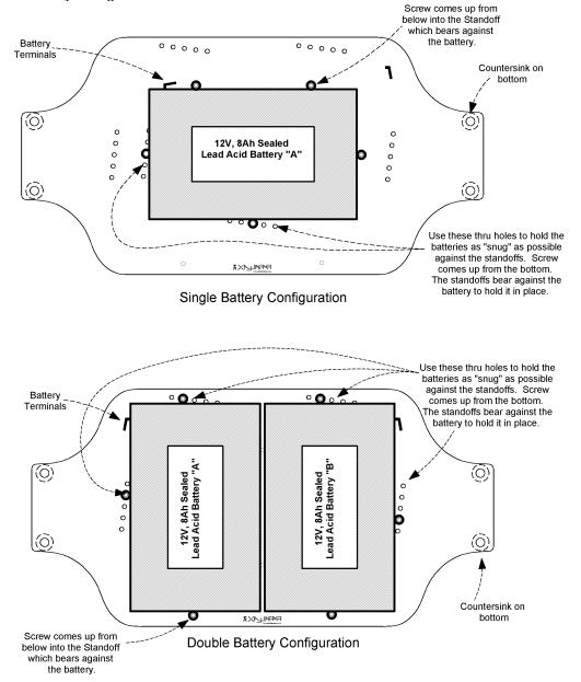
Firmly secure your batteries to the Battery Tray. Several methods can be used, including zip-ties or double-sided sticky tape. If you're using a standard 12 V, 7.5 Ah sealed lead acid (SLA) Battery, the (included) 5/8" F/F standoffs and #4-40 x  $\frac{1}{2}"$  long pan-head screws can hold your battery securely as shown. The staggered hole patterns accommodate slight dimensional variances between different brands of batteries.
