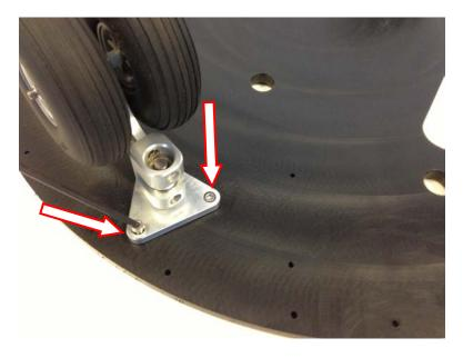
Insert a  $\#6 \times 3/8"$ , Socket-head cap screw included with the Caster Wheel Kit Rev B into each mounting hole in the caster's mounting plate. Tighten using the included ball end hex key for this operation.
