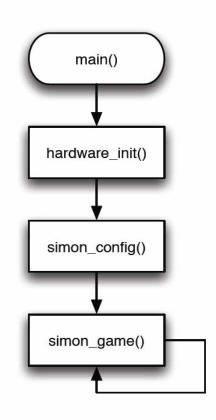
After all configuration is complete, we move into the core simon\_game() routine. Immediately after entering simon\_game(), the system is configured to enter a low-power sleep mode and to awake on a button press from any of the four buttons. Sleep mode is attained by calling a specific sequence of functions/macros, which define the type of sleep mode we want to enter, configuring the interrupts, and then going to sleep:
