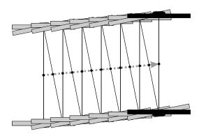
The illustration shows another consequence of this point of view: the tendency of the computed path to "crab" in a direction opposite the side that took the first step. If both wheels were turning simultaneously, this would not be happening. Even though the angle of each step is exaggerated here, it is still something we need to address later on.
