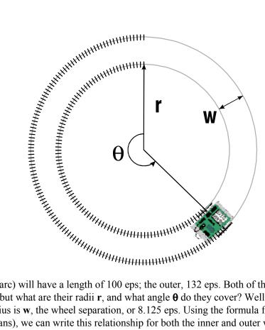
The inner track (arc) will have a length of 100 eps; the outer, 132 eps. Both of these tracks have a common center, but what are their radii r, and what angle **0** do they cover? Well, we know their difference in radius is w, the wheel separation, or 8.125 eps. Using the formula for arc length  $D = r \theta$ (**6** here is in radians), we can write this relationship for both the inner and outer wheel, as follows:
