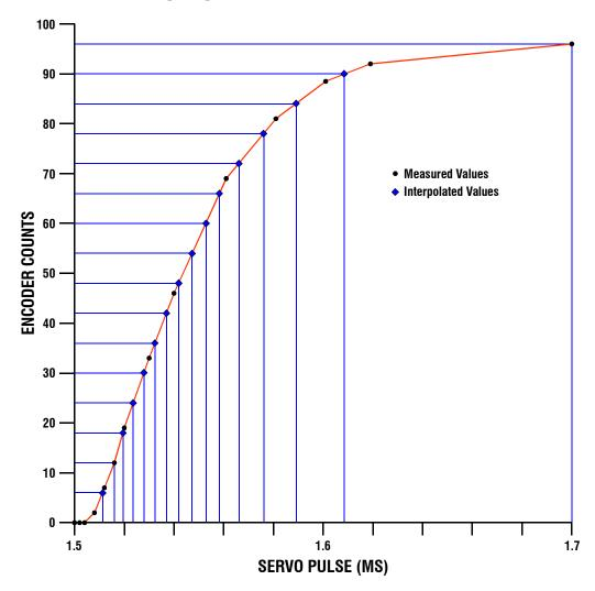
Once the interpolated pulse widths for sixteen equally-spaced velocities are obtained in each direction for each servo, they are written to the BASIC Stamp's EEPROM in the first 64 bytes. The byte values represent offsets from the null value of 1.5ms and are scaled appropriately for the BASIC stamp version being used.
