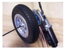
Step 12: Attach the Encoder PCB using two # 4-40 x 1/8" flat head Philips screws, as shown.
