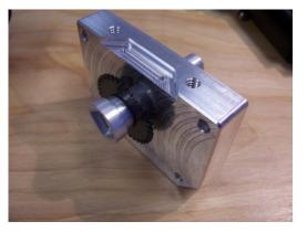
**Step 3:** Insert the motor shaft into the large diameter end of the drive axle.
