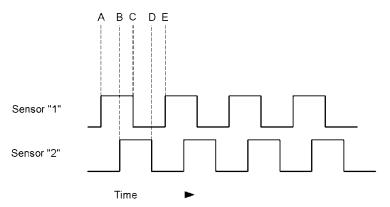
In the diagram, notice that after sensor 1 goes high (A), sensor 2 then goes high (B) as the encoder continues to rotate. Then, as the encoder continues to spin, sensor 1 goes low (C), and then sensor 2 follows (D). Because sensor 1 went high before sensor 2 (A-B), this indicates that the encoder disk is rotating in one direction (in the case of a robot, either forward or reverse). If sensor 2 went high before sensor 1, then the disk is rotating in the opposite direction.
