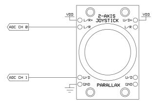
This circuit creates two voltage dividers referenced to VDD (in this case 5 V), using a 2-channel ADC (in this case the MCP3202) to read the voltages at the L/R and U/D pins using the code below. **Caution:** Do not apply voltage to the L/R+ or U/D+ pins that exceeds the I/O pin voltage rating of the device you connect to L/R or U/D, up to 10 VDC maximum. Ground<Analog voltage output at L/R and U/D<VDD.
