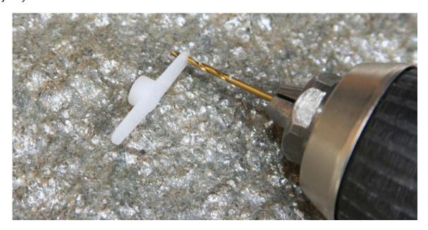
Step 10: Connect the 1/16" ball links to the servo horn
