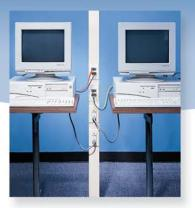
The dual-channel power and communication pole provides channel separation for the installation of communication cabling and modules, eliminating the need for two poles. One compartment is factory wired with two duplex style 20A, 125V NEMA 5-2OR grounding-type, specification-grade receptacles; leaving the second compartment for routing low-voltage cabling.
