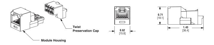
Dimensions are in inches [Dimensions in brackets are metric]
