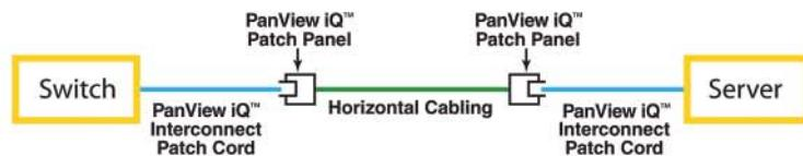
When network elements such as switches need to be reconfigured, the PanView iQ™ System provides LED guidance to ensure proper switch port allocation/de-allocation. Network elements such as servers can also be monitored at the physical layer to ensure proper connectivity. With the PViQ™ System Hardware, both ends of the switch-server relationship are monitored via the SmartZone™ Software Suite, which leads to quicker problem resolution and rapid service/application restoration.
