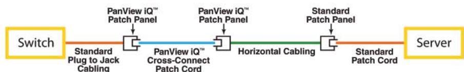
In cross-connect configurations, the highest density network element (such as the high-speed switch) is permanently cabled through the back of a PViQ™ Patch Panel with modular jacks. PViQ™ Patch Cords are then connected between the front of that panel and the remote PViQ™ Patch Panel cabled via horizontal runs to remote cabinets, typically containing other network elements (e.g., servers) or endpoint equipment (e.g., computers, IP phones, security equipment, etc.).
