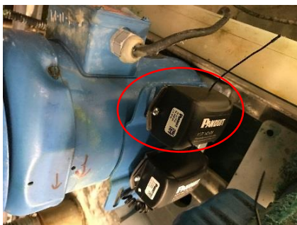
Figure 8: Sensor Magnetically Mounted to Equipment
