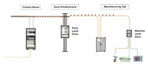
Following a zone topology with the Panduit building block architecture creates a highly scalable and flexible network deployment.
