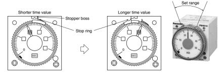
Note) The stoppers for the lower limit setting set ring and the upper limit setting set ring face the opposite directions.
