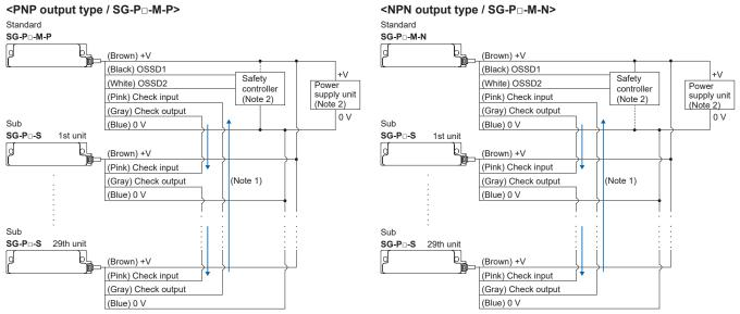
Notes: 1) For connecting multiple units in series connection connect the check output line (gray) with the check input line (pink) of the SG-P<sub>□</sub>-S sub unit connected next. Connect the check output line (gray) of the SG-P□-S sub unit connected at the end with the check input line (pink) of the standard unit (SG-P□-M-P / SG-P -M-N) placed at the beginning.
