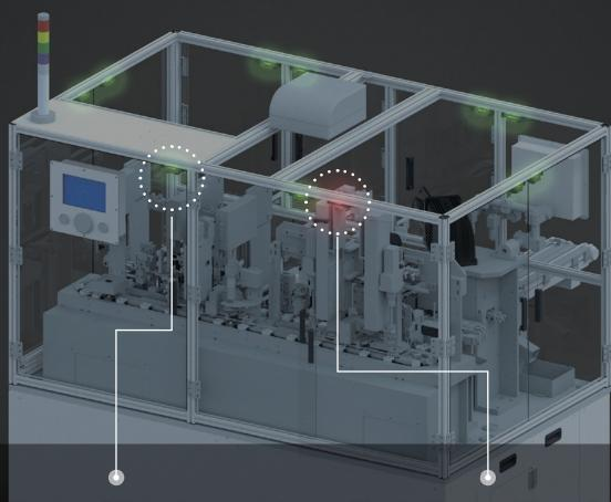
The indicator of the safety switch on the closed door flashes to notify the unsafe condition.
