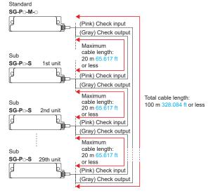
The total length of the cables connected from the SG-Pu-M-u standard unit to the last SG-P -S sub unit (farthest from the standard unit) must not exceed 100 m 328.084 ft. The cable connected from each switch body to the adjacent switch body must not exceed 20 m 65.617 ft.
