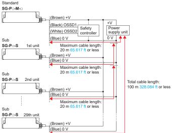
The total length of the cables between the switch bodies and power supply unit and the total length of the cables between the switch bodies and safety control unit must not exceed 100 m 328.084 ft each. The cable connected from each switch body to the adjacent switch body must not exceed 20 m 65.617 ft.
