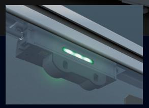
The indicators of the safety switches on all other closed doors that are interlocked with the open door flash in green to notify the unsafe condition.
