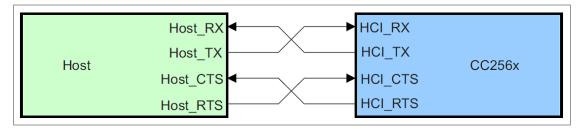
When the UART RX buffer of the CC2564C passes the "flow control" threshold, it will set the signal UART\_RTS high to stop transmission from the host.
