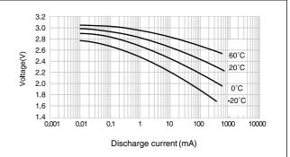
Operating voltage vs. Discharge current(voltage at 50% discharge depth)
