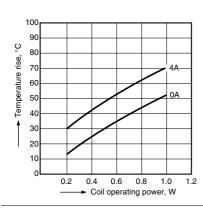
4.-(2) Coil temperature rise Tested Sample: S4EB-24V, 4 Form A
