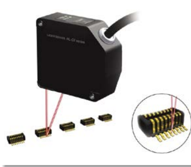
Detection of deformed narrow pitch connector leg pins
