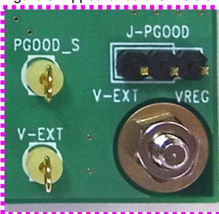
Figure 6. Appearance of J-PGOOD
