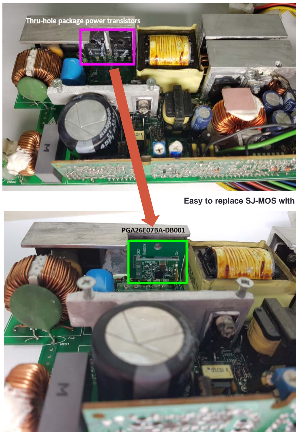
Figure 12: For illustration purpose, PGA26E07BA-DB001 is conveniently mounted on an actual power supply
