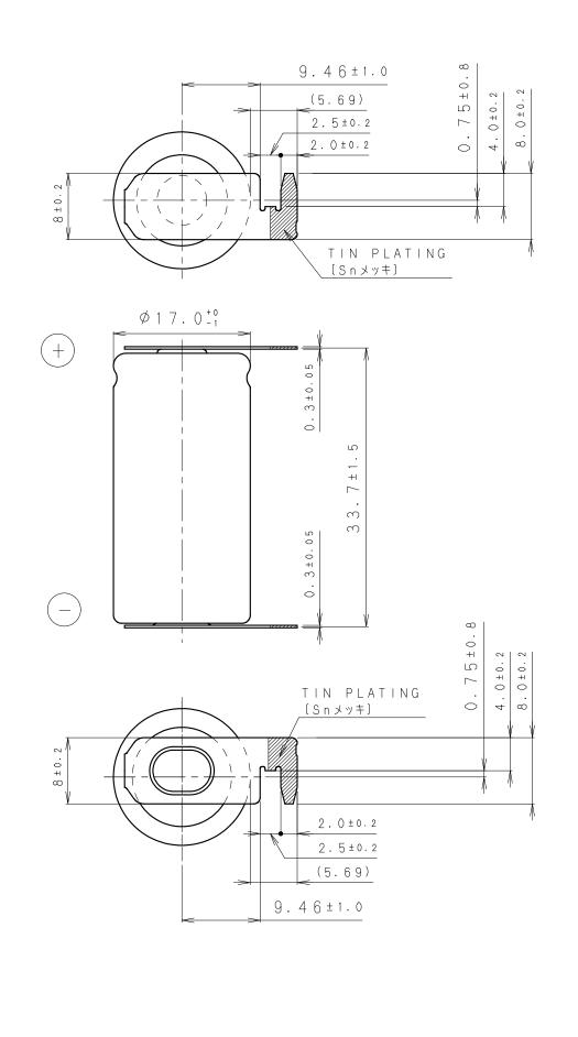
NOTE [注記] 1. NOMINAL VOLTAGE:3V[公称電圧:3V] 2. TAB WELDING STRENGTH OVER 30N [端子溶接強度:30N以上] 3. TAB MATERIAL:STAINLESS STEEL WITH TIN PLATING [端子材料:基材 ステンレス/表面 部分Snメッキ 4. ():REFERENCE DIMENSION AND ANGLE [())寸法、角度は参考値]
