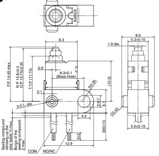
6. Wire leads type, Simulated roller lever
