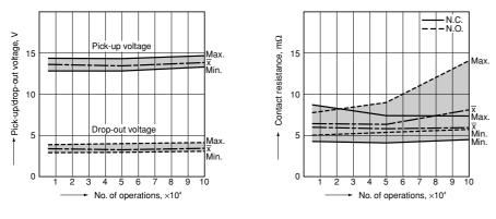
3. Electrical life (SP4, 10 A 250 V AC resistive load) Change of pick-up and drop-out voltage
