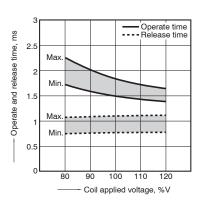
6-(2). Operate and release time (with diode) Tested sample: AGN2004H, 6 pcs.
