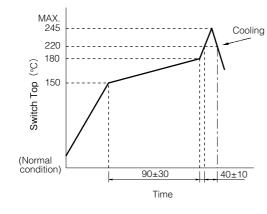
\* Reflow temperature may vary by location even in the same reflow condition. Please check the reflow temperature at terminals and at the top of a switch to make sure the both temperatures are within the specification. If even one of them is out of the specifications, please adjust.
