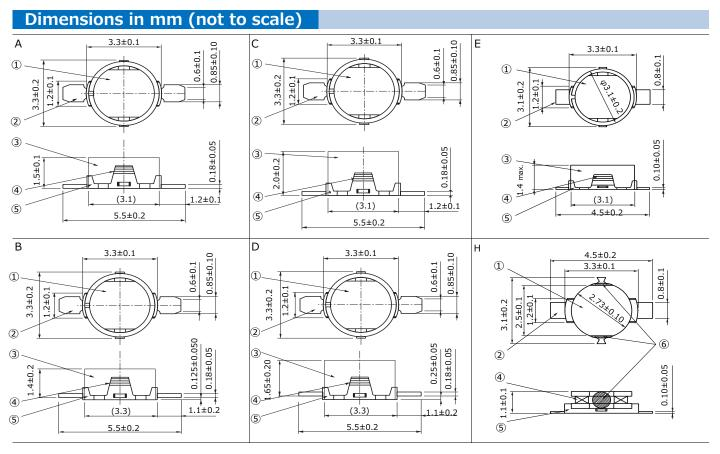
Part Name: ①Core ②Terminal ③Ring ④Coil ⑤Terminal board ⑥Adhesive
