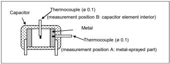
When a capacitor is sent through a high-temperature atmosphere after being subjected to the (flow) soldering process, check the mounting temperature including the temperature of the capacitor in the high-temperature atmosphere.
