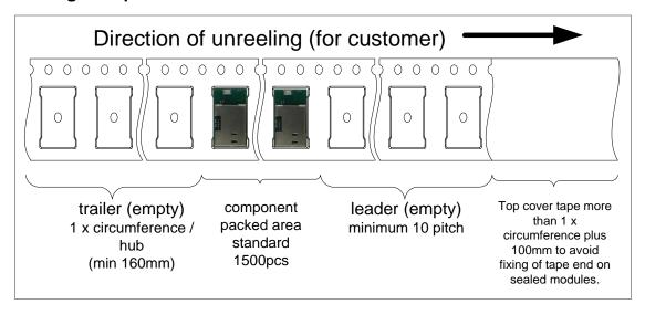
Empty spaces in the component packed area shall be less than two per reel and those spaces shall not be consecutive.
