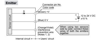
Symbols ... D: Reverse supply polarity protection diode
