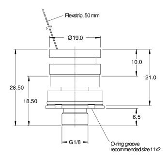
Mass: approx. 35 g A G 1/8 version with spanner flat is available on request. Please contact TE Connectivity. dimensions in mm
