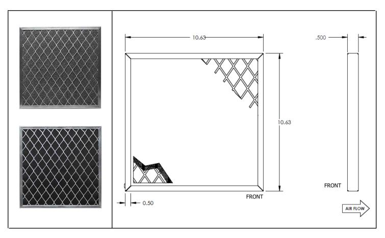
Orion Fans Hydrophobic Mesh air filters are water-repellant and offer a low pressure drop, cost-effective solution. The hydrophobic media is durable, cleanable, and moisture-resistant. Designed for outdoor cabinets, process equipment applications requiring mist elimination, or other harsh environment installations.
