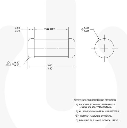
Figure 1. 2-TERMINAL, SOD-80, JEDEC DO-213AC, MINI-MELF
