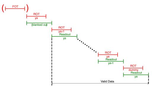
Figure 16. Integration and Readout Sequence of the Sensor Operating in Pipelined Global Shutter Mode with Zero ROT Readout.
