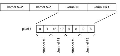
Figure 42. P1-SE: Data Output Order for 4 LVDS Output Channels in Subsampling Mode on a Color Sensor
