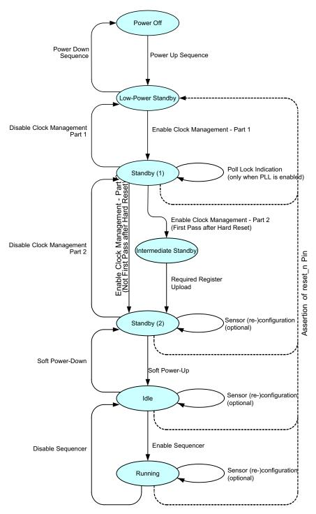
Figure 17. Sensor Operation Flowchart
