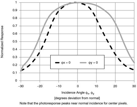
Figure 5. Central Pixel Photoresponse to a Fixed Optical Power with Incidence Angle varied along  $\phi_x$  and  $\phi_y$
