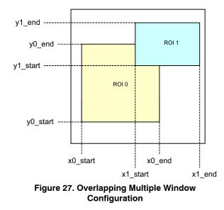
The sequencer analyses each line that need to be read out for multiple windows.
