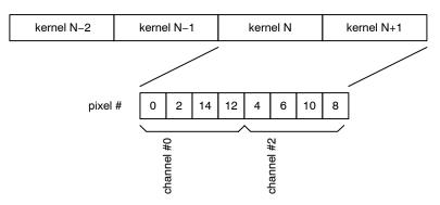
Figure 40. P1-SN/FN, P3-SN/FN: Data Output Order for 2 LVDS Output Channels in Subsampling Mode on a **Monochrome Sensor**
