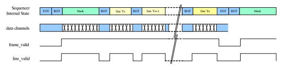
Figure 45. P2–SN/SE/FN: Frame Timing Indication
