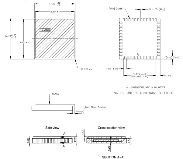
Figure 50. Package Drawing for the 48-pin LCC Package
