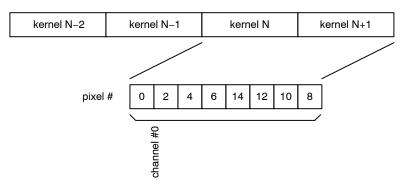
Figure 41. P1-SN/FN, P3-SN/FN: Data Output Order for 1 LVDS Output Channels in Subsampling Mode on a **Monochrome Sensor**
