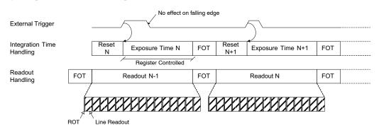
Figure 14. Triggered Shutter Operated in Master Mode
