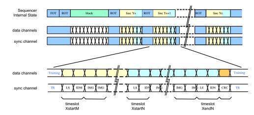
Figure 34 shows the detail of the readout of a number of lines for readout of two overlapping windows.
