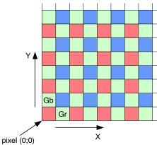
Figure 2. Color Filter Array for the Pixel Array
