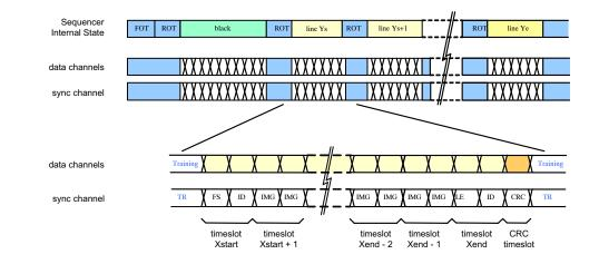
Figure 33 shows shows the details of the readout of a number of lines for single window readout, at the beginning of the frame.
