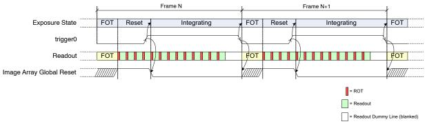
Figure 25. Exposure Time Control in Global–Slave Mode
