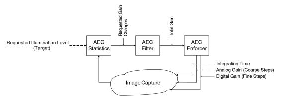
Figure 30. Automatic Exposure Control Loop
