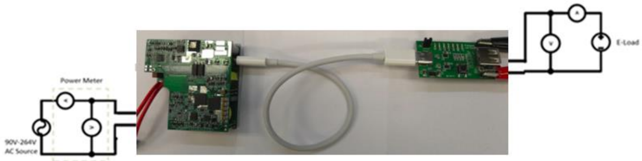
Figure 1: PD Test Setup for 90W PD/QC Demoboard
