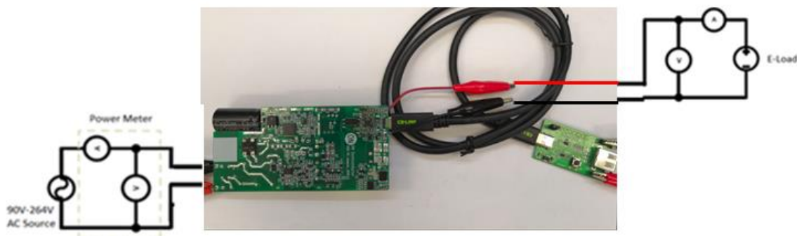
Figure 1: PD Test Setup for 90W PD/QC Demoboard
