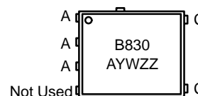
SO-8 FLAT LEAD CASE 488AA STYLE 2
