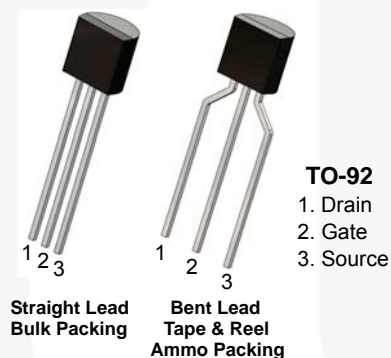
Figure 1. J175 / J176 Device Package
