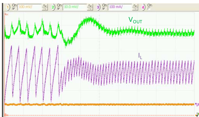
Figure 13. PFM to PWM Transition at V_{IN}=3.6V , 2 \mu s/div . Figure 14. PWM to PFM Transition at V_{IN}=3.6V , 2 \mu s/div .
