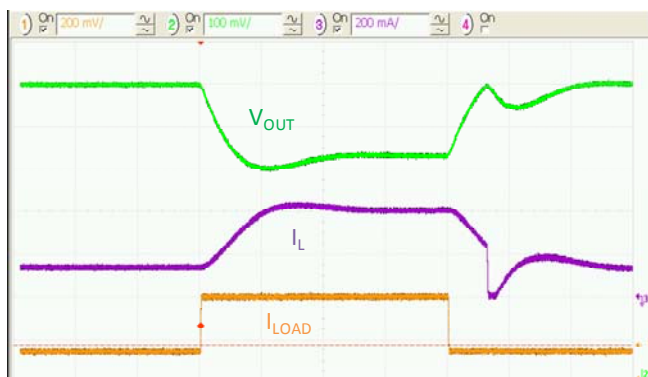
Figure 24. Load Transient 150mA to 400mA, V_{IN}=3V , t_{RISE}=t_{FALL}=100ns , 5μs/div.
