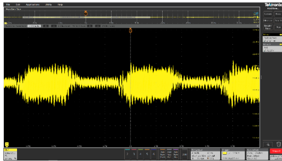
Figure 26. Transient Load on 12 V BUS
