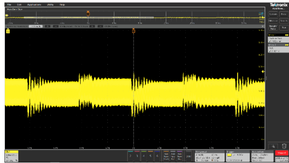
Figure 25. Transient Load on 9 V BUS
