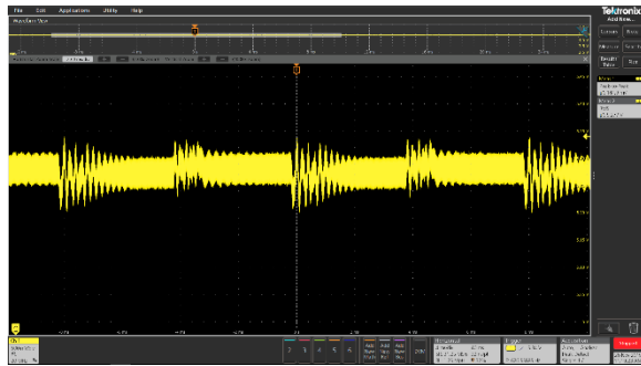
Figure 24. Transient Load on 5 V BUS
