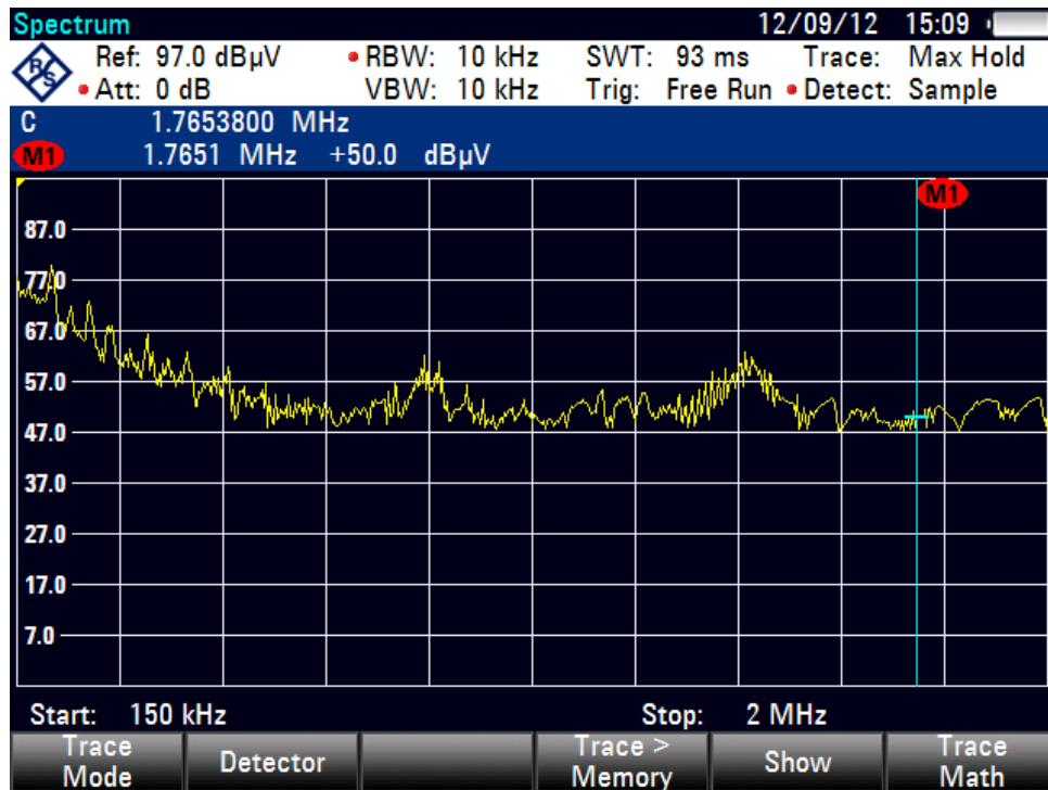
Figure 29. Conducted EMI Pre-compliance 150 kHz–2 MHz
