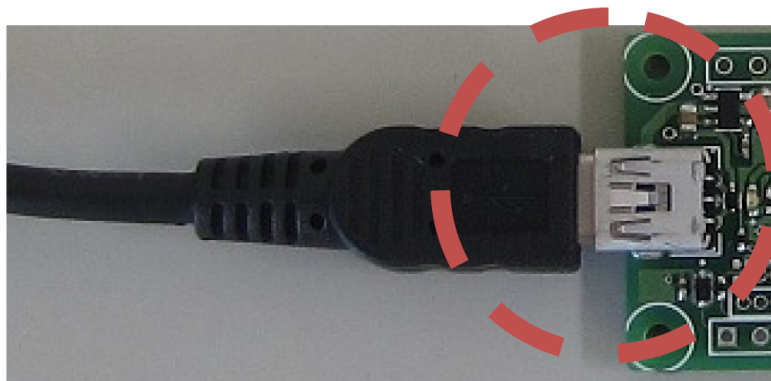
Figure 5. Connection via USB-Mini Cable
