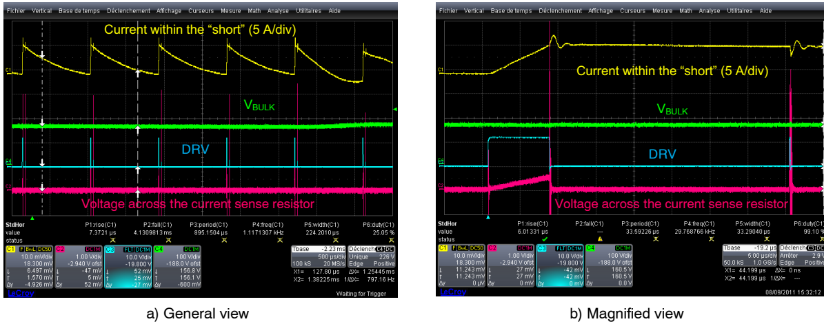
Figure 17. Shorting the Bypass Diode and the NTC
