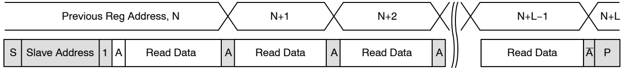
Figure 12. Sequential READ, Start from Current Location
