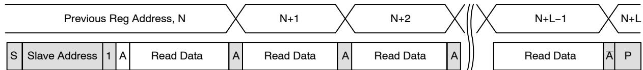
Figure 40. Sequential READ, Start from Current Location
