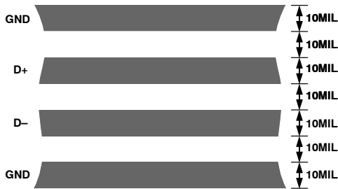
Figure 19. Arrangement of Signal Tracks
