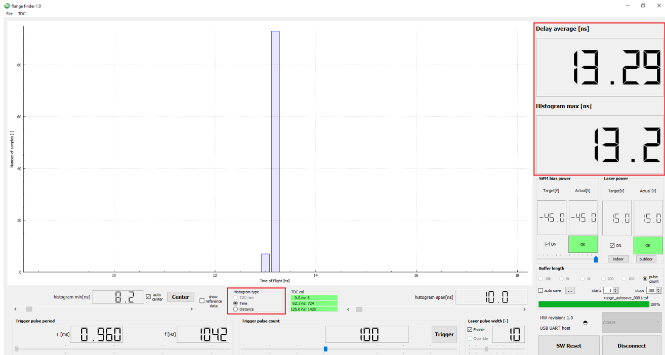
Figure 16. Switching from Distance to Time of Flight Measurement [ns]
