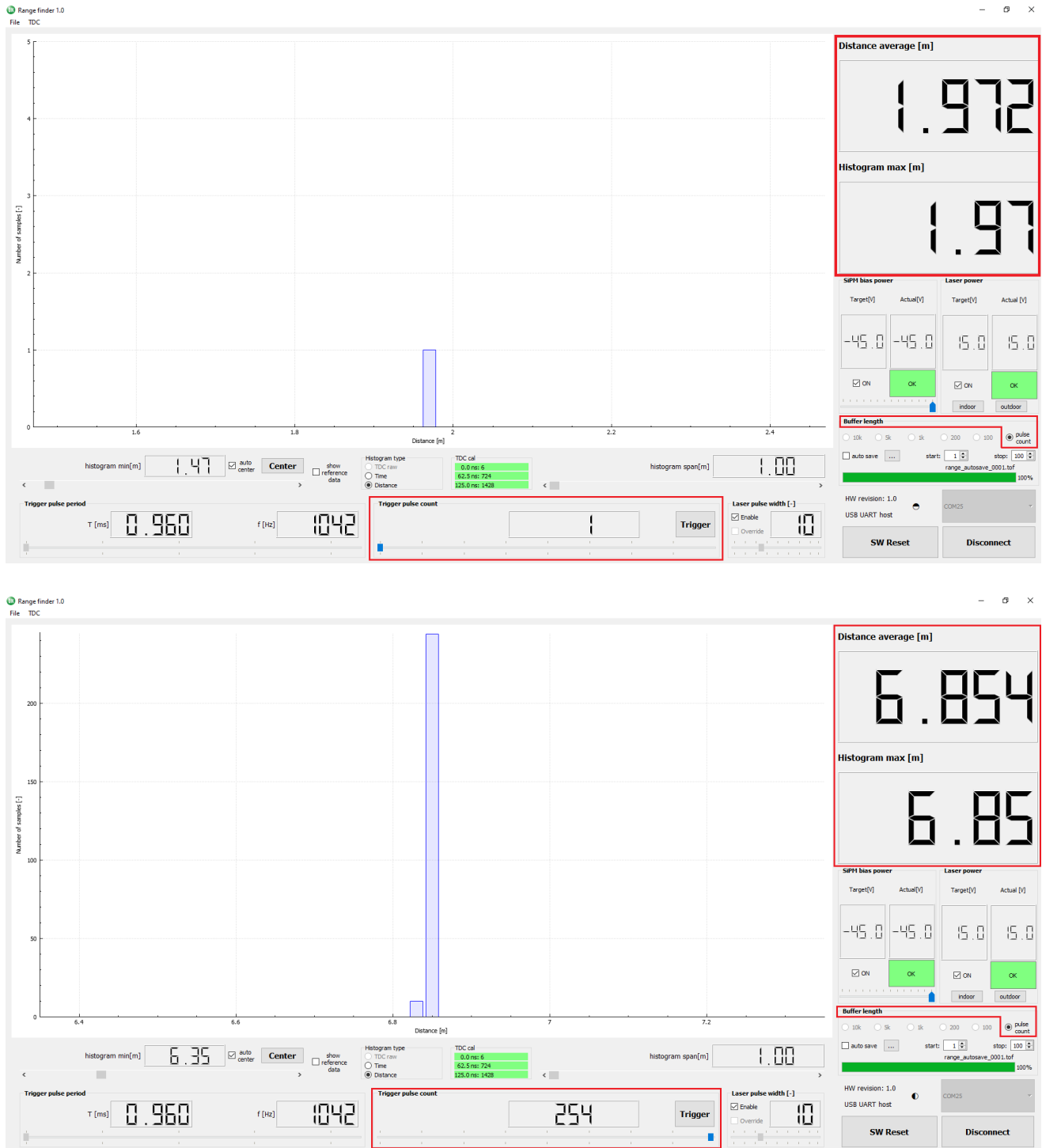
Figure 17. Trigger Pulse Count can be Adjusted between 1–254 Pulses
