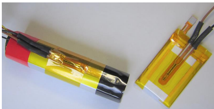
Figure 7. A LEAD TYPE THERMISTOR MOUNTING
