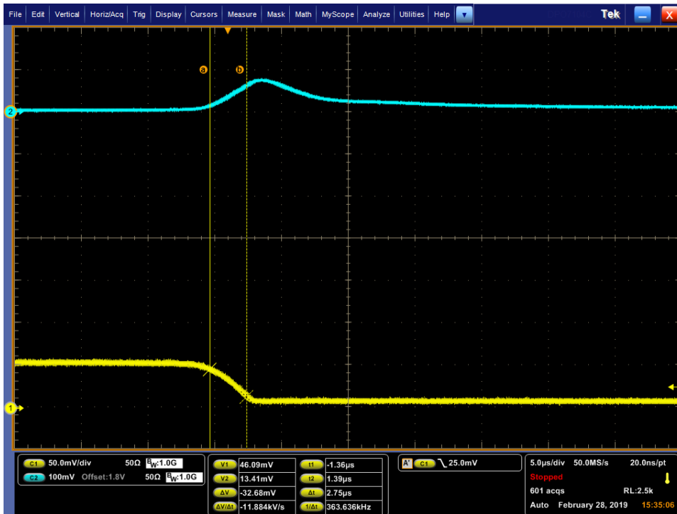
Figure 6: Load step from 125mA to 0A at 10kHz frequency.
