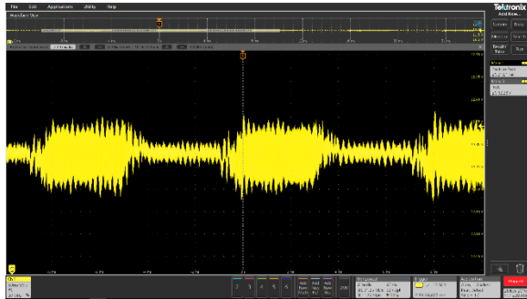
Figure 20 - Transient load on 12V VBUS
