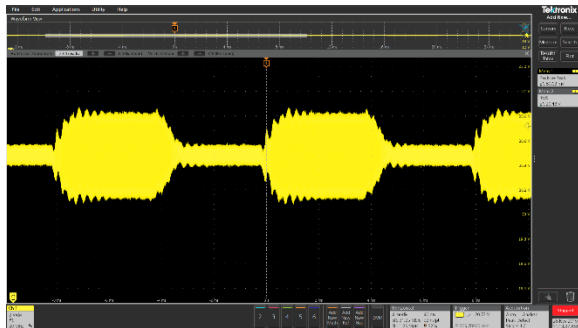
Figure 22 - Transient load on 20V VBUS
