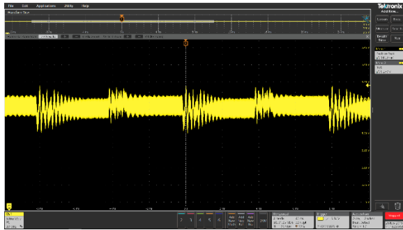
Figure 18 - Transient load on 5V VBUS
