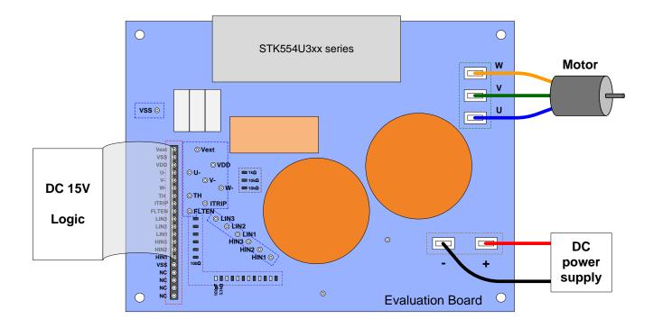
**Step1**: Please connect HIC, each power supply, logic parts, and the motor to the evaluation board,
